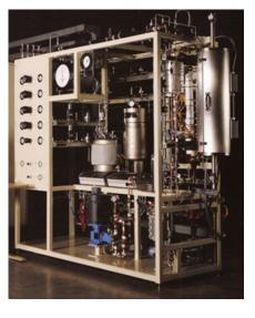
Option 1 | Packed Tube Reactor Option 2 | Gradientless Reactor Maximum System Pressure | 100 bar or 200 bar Maximum Reactor Temperature | 500 °C Catalyst Capacity | 50 mL Gas Delivery Modules | Two (2) Low Pressure Nitrogen | One (1) Gas Feed Rate | Up to 1200 SLPH Liquid Delivery Module | Two (2) Liquid Feed Rate, Standard | 3-600 mL/hr Liquid Feed Rate, Optional\* | 0.6-300 mL/hr Standard Materials of Construction | 3165S
